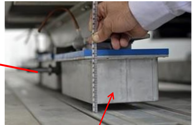
Superconductors refrigerated with \text{LN}_2 inside of cryostats
