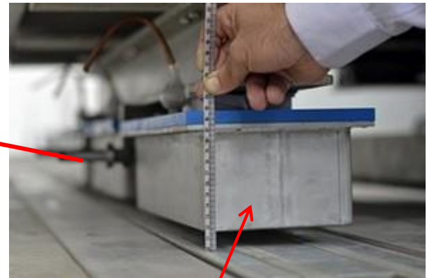
Superconductors refrigerated with LN 2 inside of cryostats
