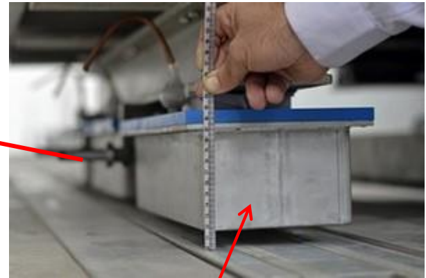
Superconductors refrigerated with \text{LN}_2 inside of cryostats
