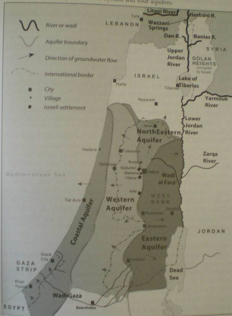
Figure 3.1 Transboundary surface water and groundwater resources of Palestine and Israel: Jordan River System and four aquifers.
