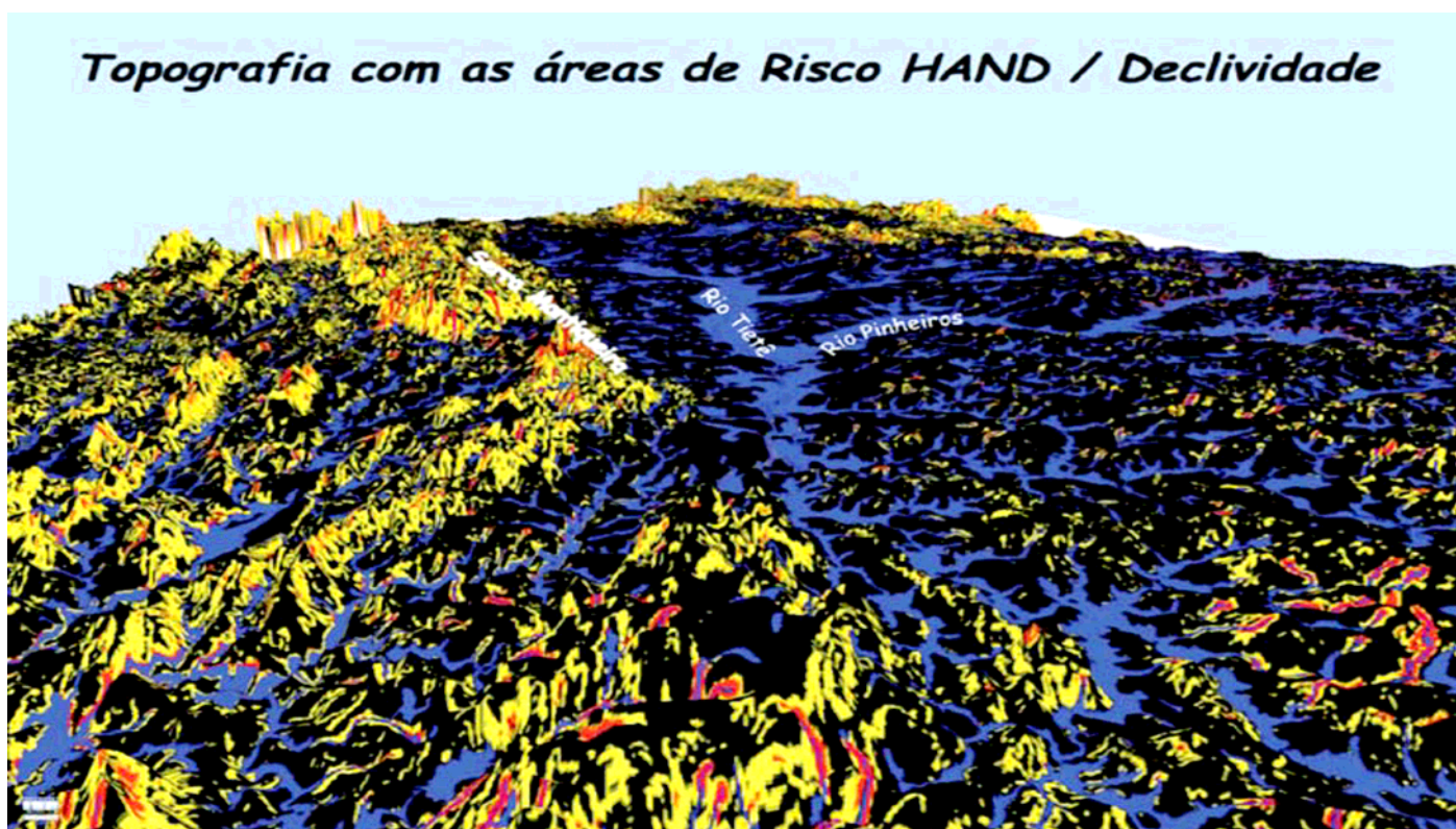
Figure 7. Use of the HAND Model to map the zones of environmental risks of the metropolitan region of São Paulo, showing in blue the areas subject to floods and flooding and in yellow (high risk) and in red (critical risk) areas subject to landslides and mass flow. In black are the areas relatively safe for human occupation. Source: Nobre et al. (2010).
