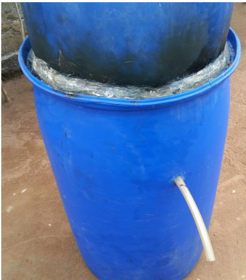
Figure 2. Base of the home made digestor
