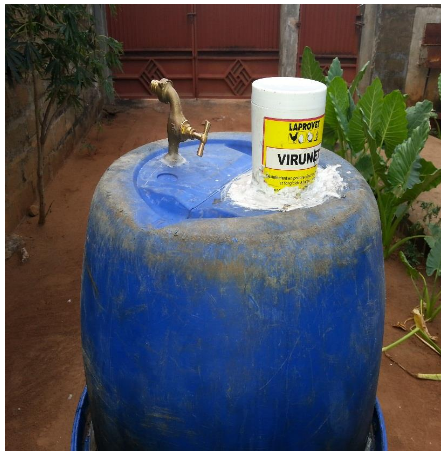
Figure 3. Lid of the home-made digestor
